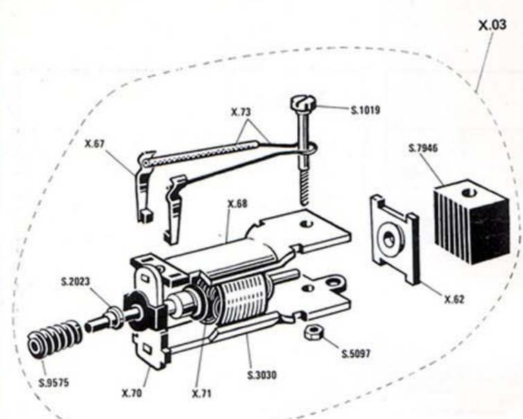
To improve control of locomotives the X.03 electric motor/driving wheels reduction ratio has been increased to 28 to 1 as compared with the 20 to 1 reduction on the older X.04 motor (Service Sheet No.81A). This improvement has been achieved by fitting the X.03 with a Single Thread Worm and the locomotive chassis with a matching 28 tooth Worm Wheel whereas the X.04 motor has a Twin Thread Worm and the older locomotive chassis a matching 40 tooth Worm Wheel.
