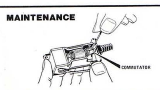
With use, carbon from the brushes will accumulate in the commutator slots. These must be cleaned regularly as shown, using a pin or sharpened matchstick.
